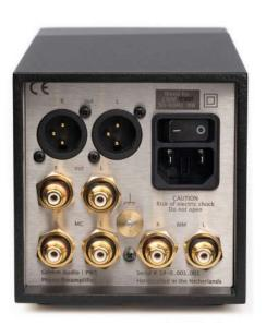
For the PW1, Peter managed to develop a solid state phono preamplifier that challenges his best tube based designs. Since harmonic distortion on LP's is quite high by nature, THD requirements were modest and he could focus on minimizing the amount of active components while optimizing their 'electric environment' in conjunction with each other. The power supply was an integral part of the design. Needless to say that passive components like capacitors and resistors were carefully picked too.
