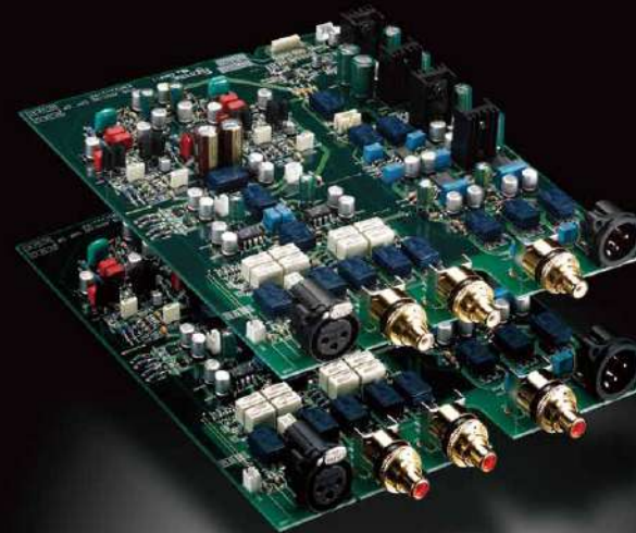
Fully balanced, dual mono audio boards
